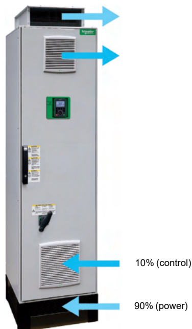
Cooling system with two separate air flows
